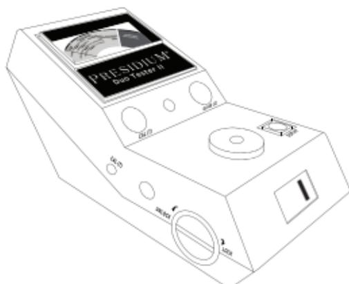
Depress the probe pen against the “CAL” disc and ensure that the probe tip is fully depressed and retracted into the housing of the probe pen. Please ensure that your fingers are touching the metallic chrome area of the probe pen. The needle indicator will calibrate to the red “CAL” strip automatically. The buzzer will beep twice upon completion of “CAL” Calibration.
