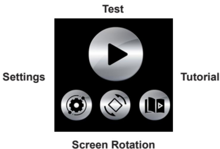
To activate a function, use finger to press any of the function on screen to activate them. To return back to the previous page, press the power button.
